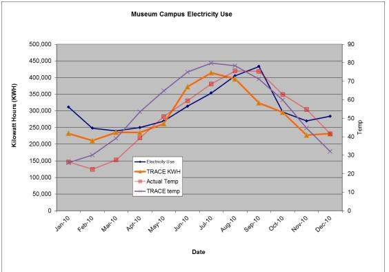
Figure 7 - Comparison of Model to Actual Energy Usage
