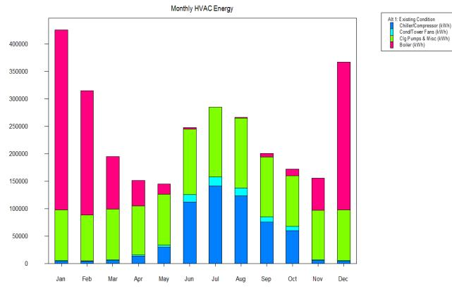
Figure 4- Monthly HVAC Energy Breakdown
